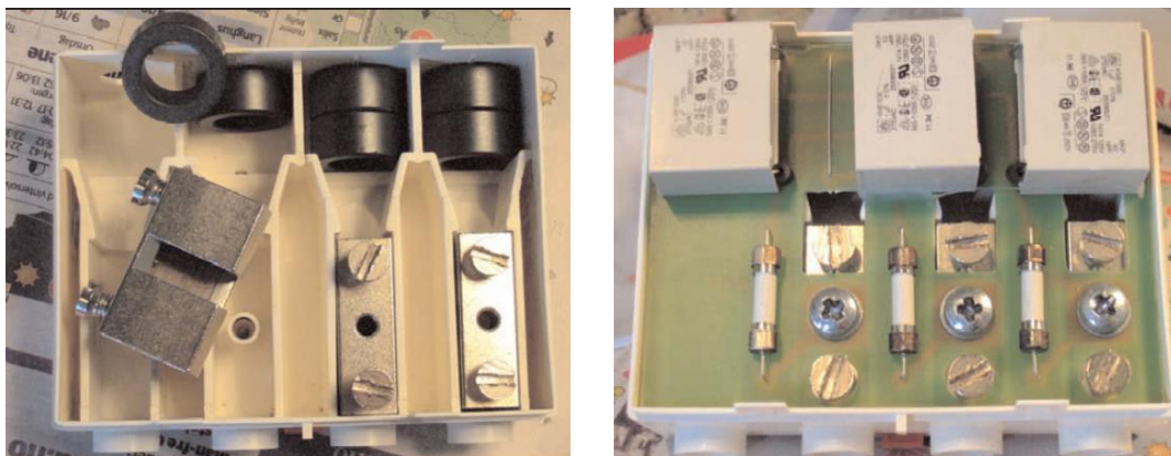
Figure 62: The Nobø Filter, the ferrite part on the left and the capacitor and fuse part on the right.
